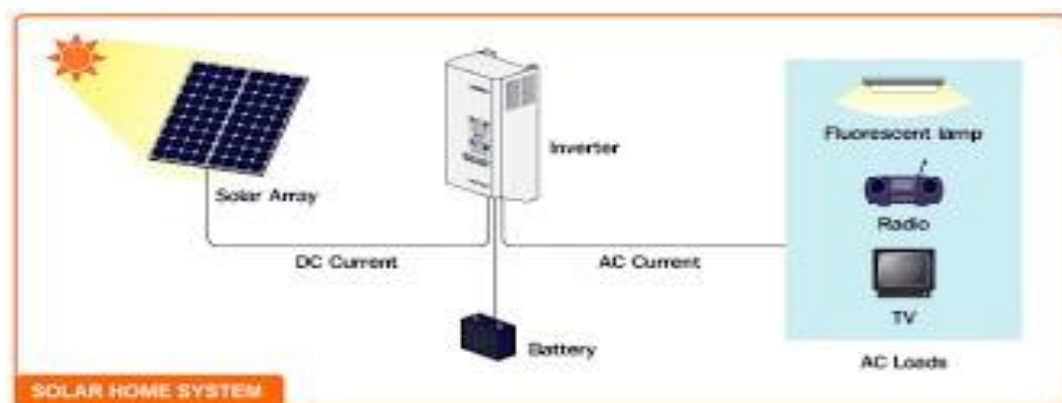
Figure 1: Solar home system with components
