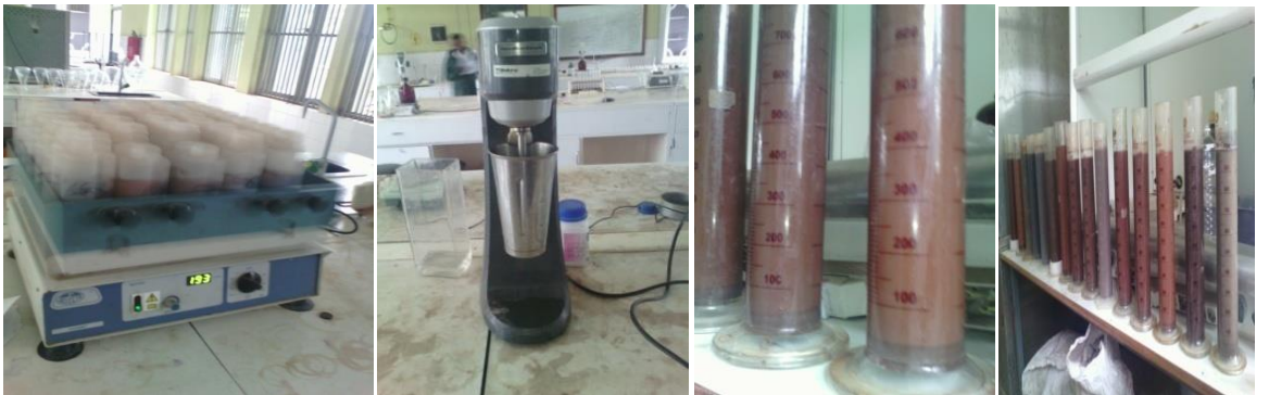
Determination of soil texture (photo by Tadewos Tesfaye on Feb, 2018).
