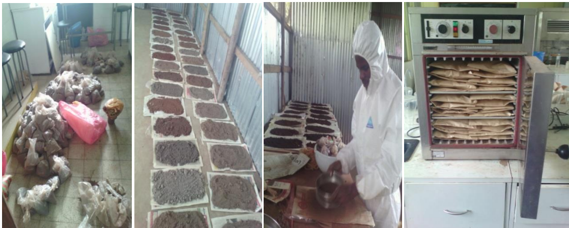
Soil preparation for SOC, soil pH, texture and Drying soil for BD determination (photo by Tadewos Tesfaye on Feb, 2018).
